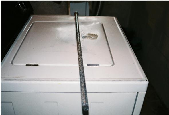
**3-month inspection of anode rod. There was the formation of the jelly substance on the anode rod which we typically see. Also decay was significant over the one month inspection.**
